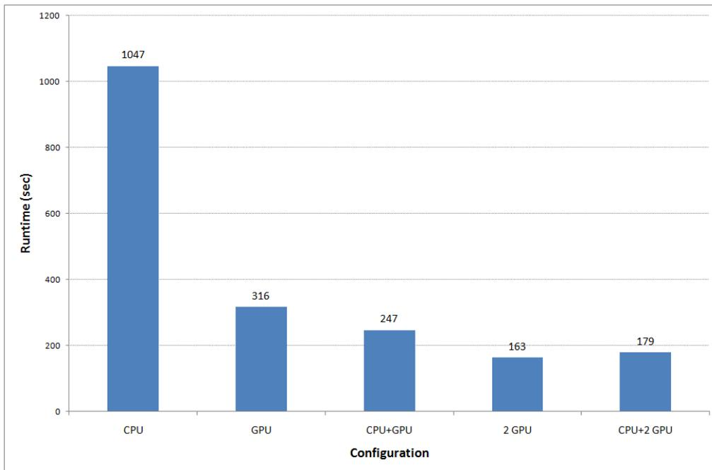
*Figure 3: Average runtime for different configurations in case of full sized images (8192x8192 pixels) using recommended tile size (2048x2048 pixels).*
