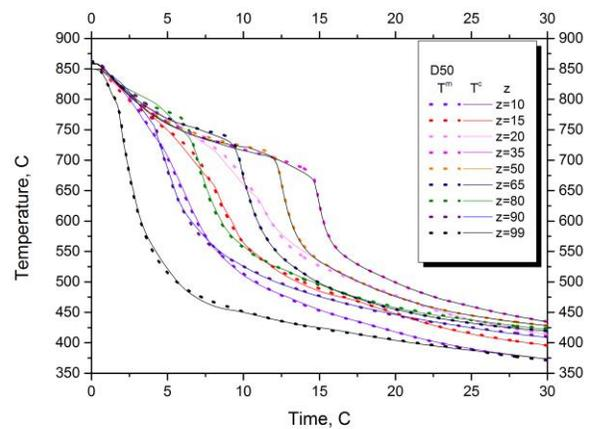
Figure 4. The measured  $T_k^m$ , and the reconstructed  $T_k^c$  cooling curves at the locations of the TCs ( $k=1,2,...10$ )
