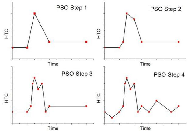
Figure 3. The concept of the sequential hybrid estimation process
