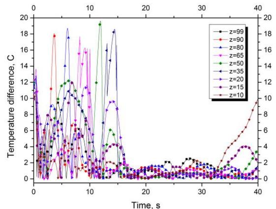
Figure 5. Difference between measured and calculated cooling curves at the locations of the TCs ( $k=1,2,...10$ ) as a function of time
