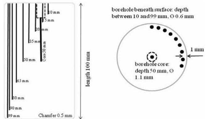
Figure 1. Locations of TCs mounted in the cylindrical work piece (produced in the IWT - Stiftung Institut für Werkstofftechnik)
