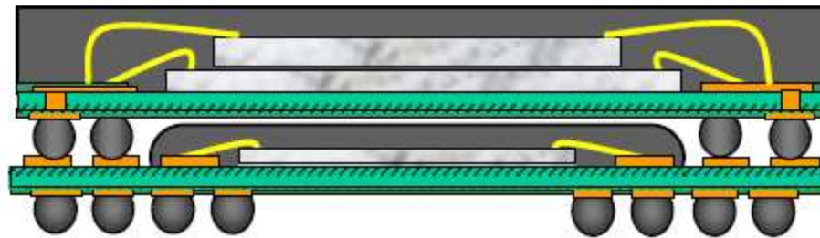
Figure: Possible PoP structure for implementing a baseband or application processor and two memory dies [13]
