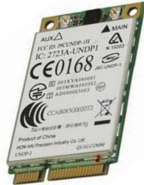
Figure: Qualcomm's UNDP-1 mini PCIe module providing wireless connectivity for laptops [36]
